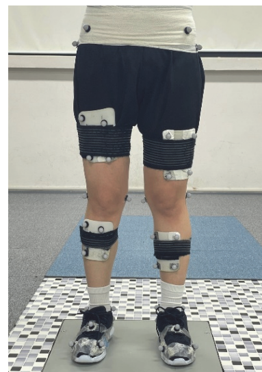
Fig. 2. Retroreflective and four-cluster markers set to obtain 3D pelvic kinematic data during dynamic walking condition.
