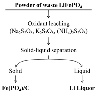
Fig. 1. Experimental procedure for the Li separation/recovery of waste \text{LiFePO}_4 powder.
