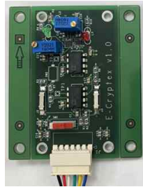
Fig. 6 PUF implementation on PCB.
