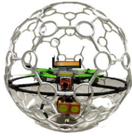
Fig. 7. Drone equipped with Air pollution measurement module
