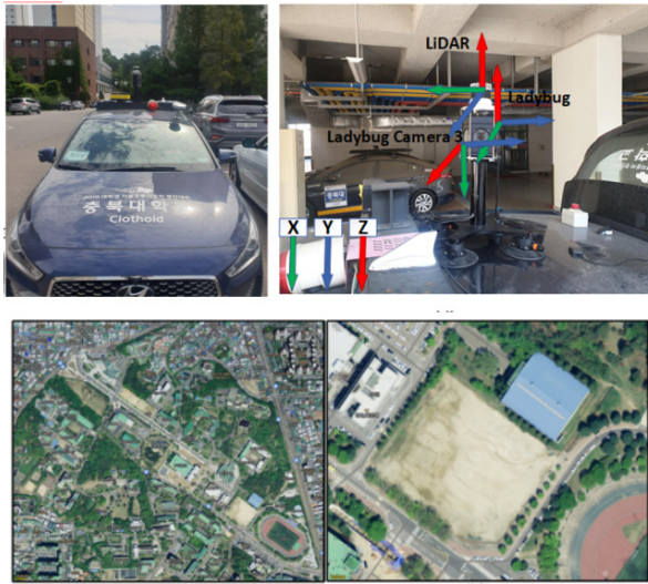
[Fig. 2] Experimental setup, Top images shows the platform used while recording. While bottom image show the data recorded region in campus
