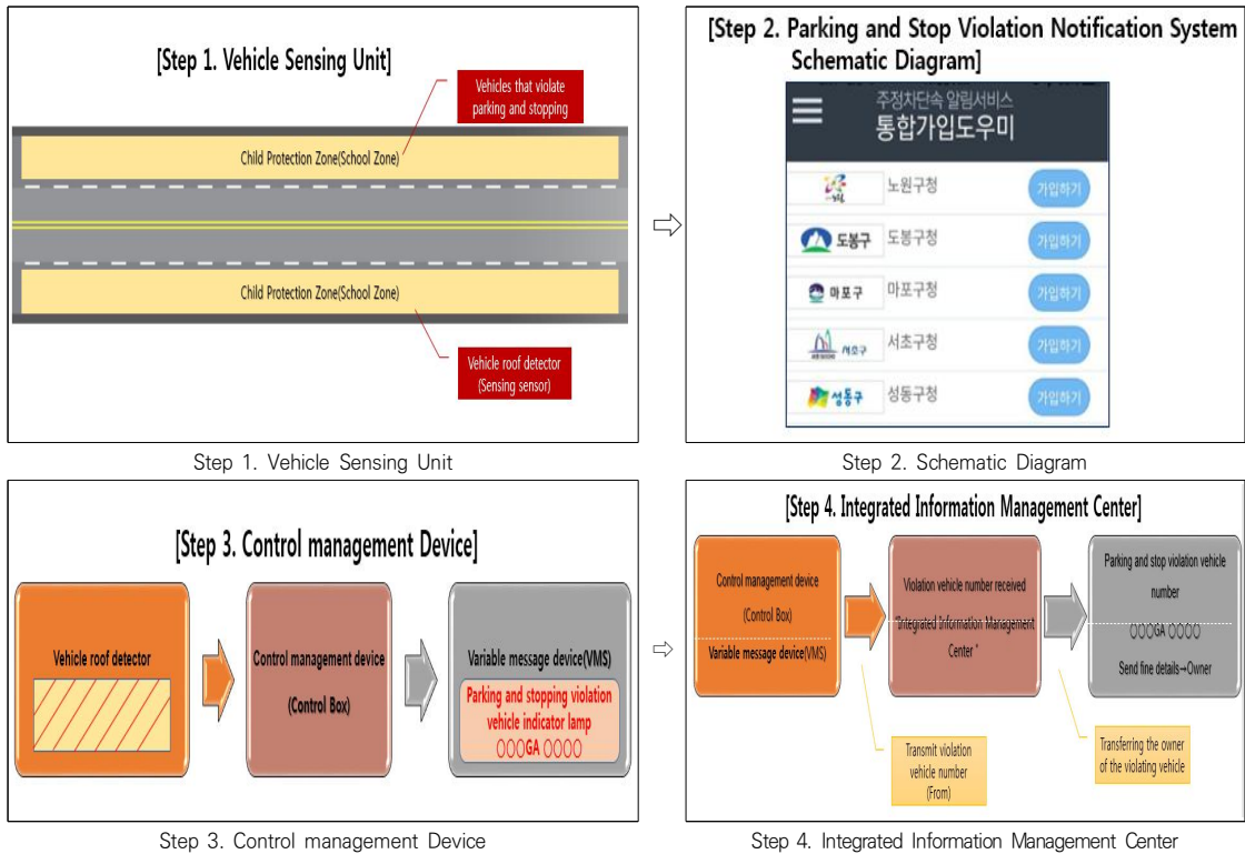
Fig. 2. Schematic Diagram & Composition Diagram of a step-by-step Parking and Stop Prevention System
