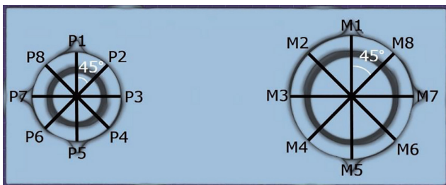
Fig. 5. Margin points for each abutment. Sixteen margins per specimen were measured. Based on the center of the abutment, the margin was set to be 45° different from the adjacent margin. Margin points in the premolar were set in clockwise order, and margin points in the molar were set in counter-clockwise order.
