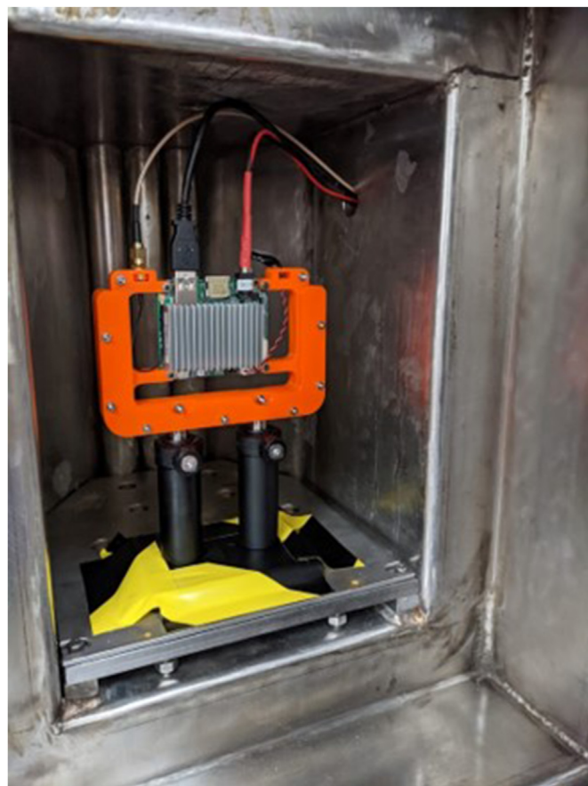
Fig. 3. DUT located in the irradiation chamber with external connections to WiFi, USB, and power from left to right at the top of the unit. The locations of the three Cobalt rod sources when in operation are visible to the rear of the chamber.
