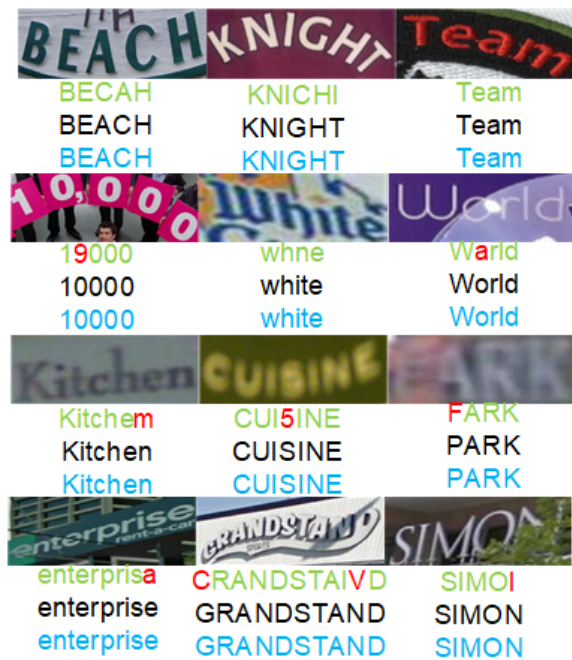
Fig. 8. Visual recognition results in two models. ASTER, RBN-STR, and Ground Truth are represented by green, black, and blue fonts, respectively. The error results are noted by red fonts.
