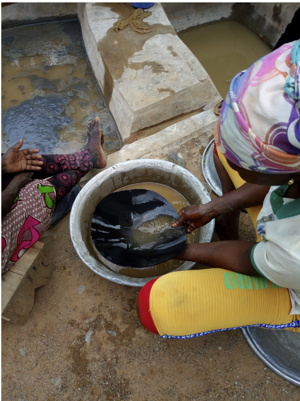
Fig. 2. Application of mercury for amalgamation without the use of PPE. Source: Fieldwork, January–June 2018
