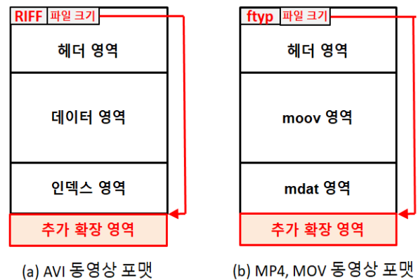
Fig. 3. Internal Structures of AVI, MP4 and MOV Video File Formats
