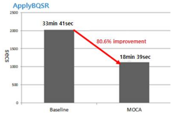
Fig. 11. Comparison of SSD and MOCA execution time and IO performance in ApplyBQSR: SSD vs MOCA
