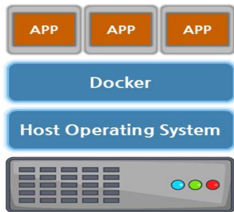
Fig. 2. System architecture of docker container systems
