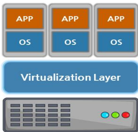
Fig. 1. System architecture of virtualization systems
