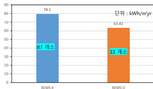
Figure 15. Primary energy consumption according to BEMS installation
