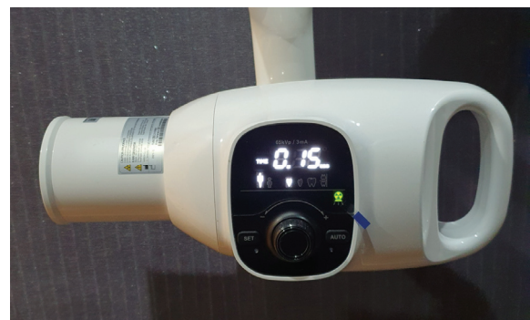
Fig. 2. Vatech's VEX-S300C dental radiography system used in the simulation. X-rays were generated under irradiations of 65 kVp, 3 mA, and 0.15 sec.
