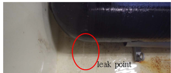
Fig. 10. RM-S1-280 cylinder low temperature test result
