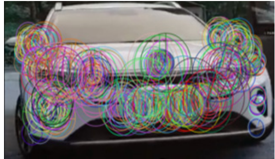
<Figure 6> Example of extracting feature points for incoming vehicles
