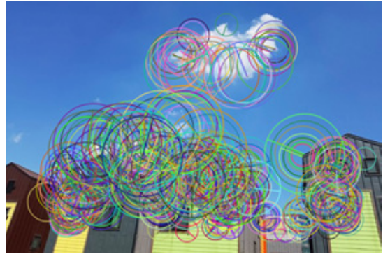
<Figure 2> Example of feature point extraction(신백균, 2020)
