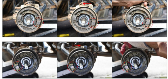
Fig. 9 Operation inspection of front wheel brake system
