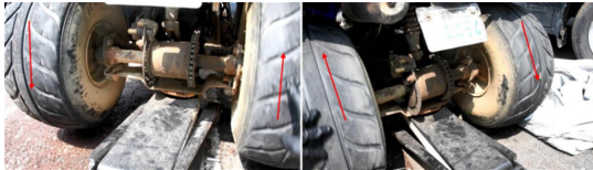
Fig. 7 Operation inspection of differential system
