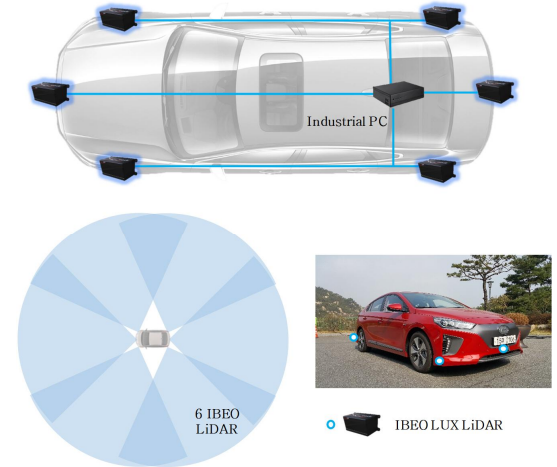
Fig. 1 IBEO LiDAR sensor configuration diagram of autonomous test vehicle
