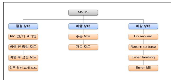
[Figure 11] UAV state mode Diagram
