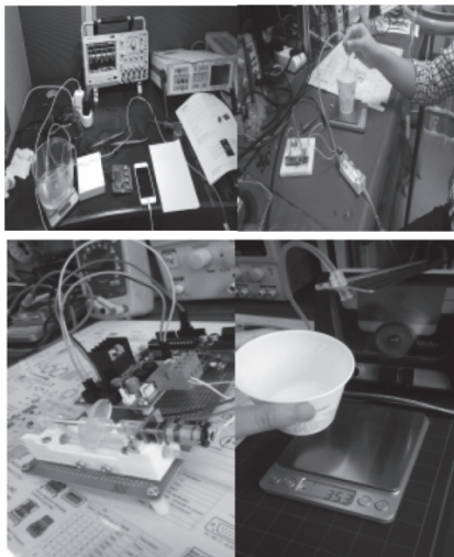
Fig. 6 Configuration of fluid discharge experiment using a fine scale (±0.1g)
