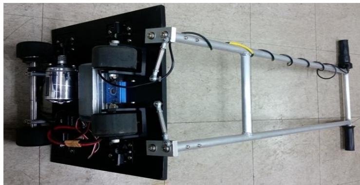
Figure 8. Prototype of 4-wheel electric scooter with 2-shafts steering system
