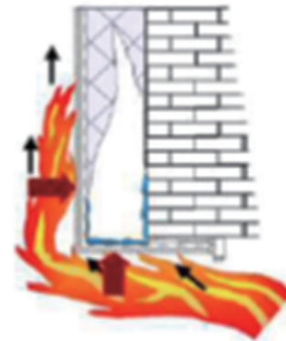
Figure 6. Flame extending from inside of building
