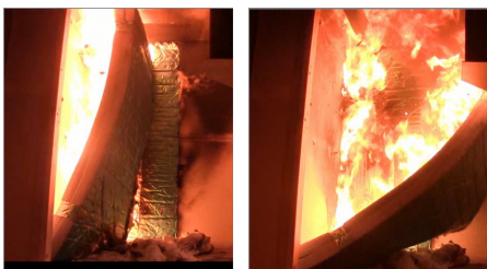
Figure 5. Insulation layer detachment due to adhesive losing mechanical strength under elevated temperature condition
