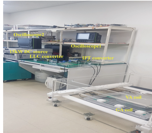
Fig. 16. Wireless charging system test pad.
