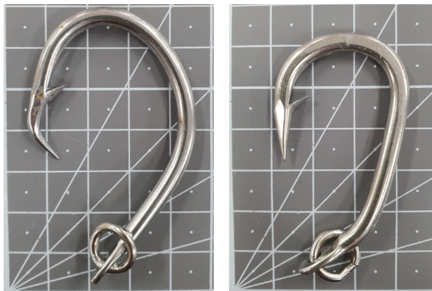
Fig. 1. Hook type used in the Korean tuna longline fishery. (left) Circle hook (C14), (right) Japanese tuna hook (3.4 sun).
