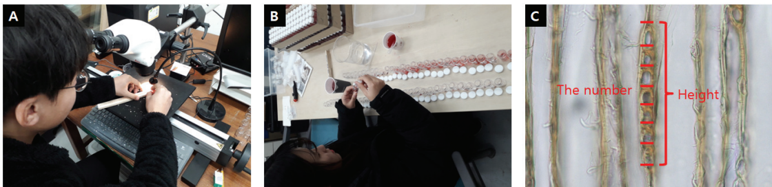
Figure 1. Sample preparation for the measurement of tracheid length and uniseriate ray height. (A) Splitting tree rings in longitudinal direction considering earlywood and latewood. (B) Staining tracheids in Safranin. (C) Measuring uniseriate ray height and counting uniseriate ray number.
