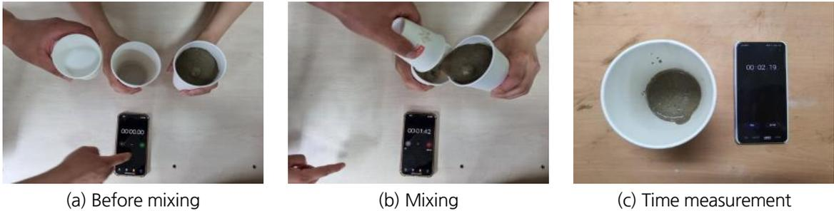
Fig. 4. Gel time test
