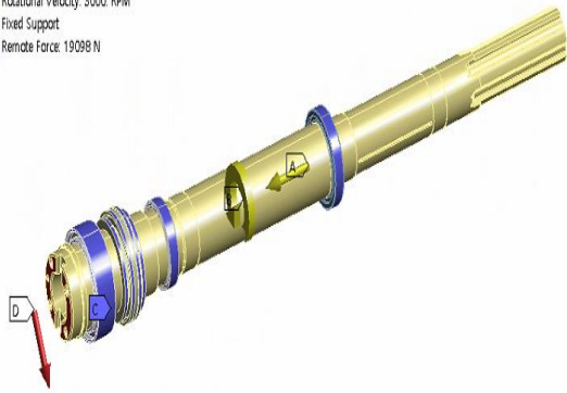
Fig. 7 Boundary and force condition of the main spindle for transient analysis
