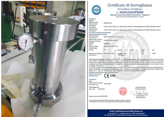
Fig. 13 Hydraulic pressure test and certificate
