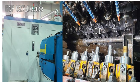
Fig. 2 HNP-627 and experimental set-up
