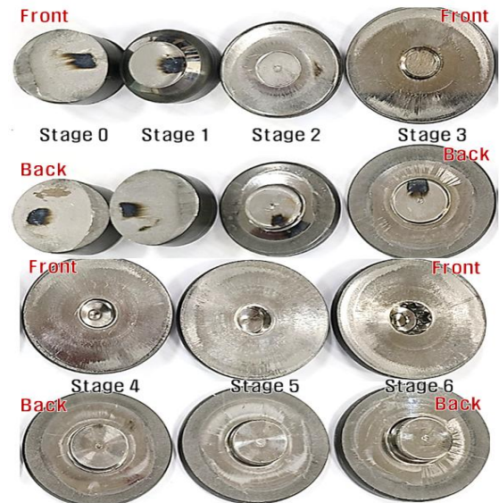
Fig. 10 Stage 0~6 Cold forging process product
