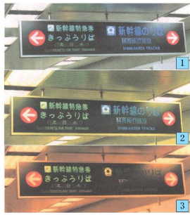
Fig. 4. Visual Change in the Yellowing Color of the Lens
