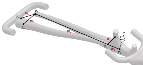
[Fig. 6] The radioulnar joint: coordinates of attachment positions of wires and constraint wrenches by the wires
