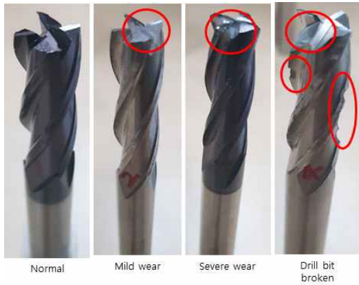
Fig. 2. Condition of the tools used in the experiment
