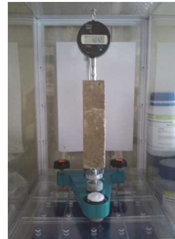
Fig.3 Length change test over time
