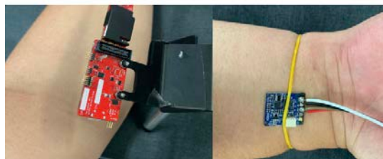
Fig. 4. Actual measurement scenarios (Left: Radar / Right: Contact sensor)
