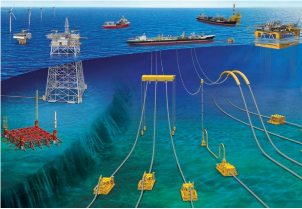
Fig. 1. Offshore platforms and subsea pipelines according to water depth (www.oilstates.com).
