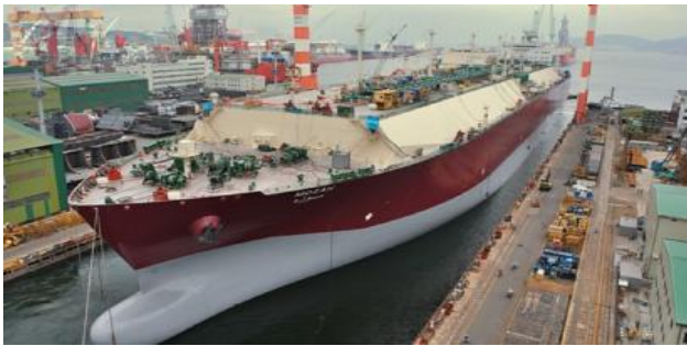
Fig. 1. Launching vessel in the dry dock. ( http://www.koreatimes.co.kr )
