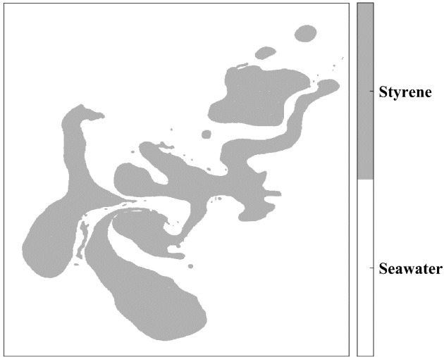
Fig. 6. Spatial distribution of styrene detection results based on spectral distance similarity (SDS) index.
