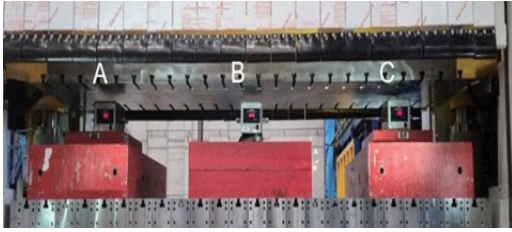
Fig. 4 Installation of press test equipment
