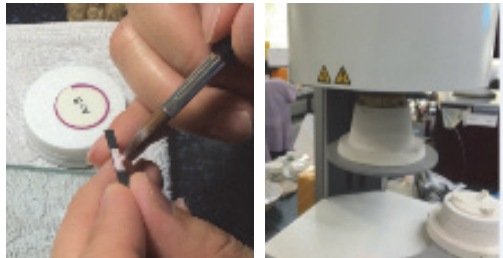
Fig. 9 Ceramic powder veneering and firing process
