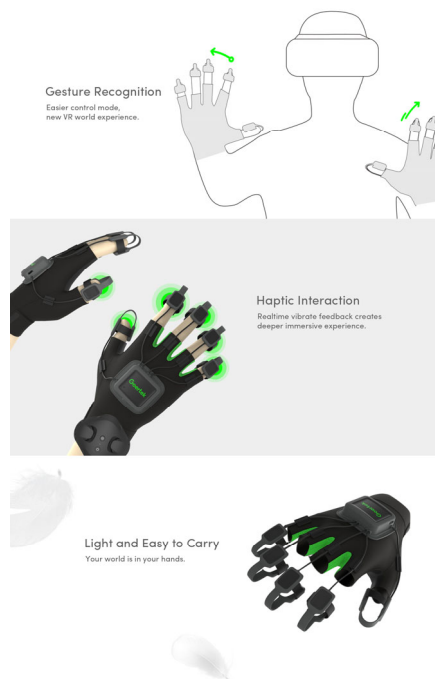
Fig. 3 Data Glove for Gesture Recognition [43].
