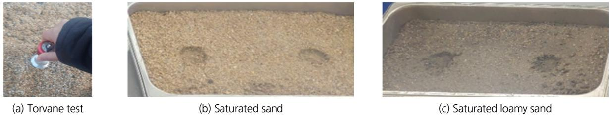
Fig. 2. Torvane test of saturated sand and loamy sand used on sheet erosion by rainfall simulation
