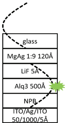
Fig. 1. Schematic diagram showing the micro cavity effect in a TEOLED.
