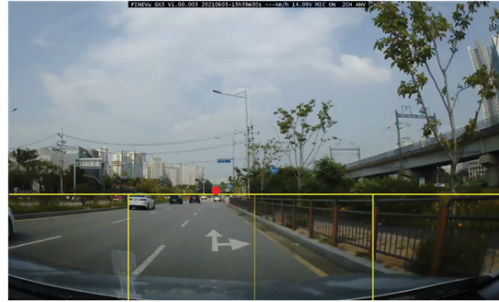
Fig. 2. ROI of an acquired image, which are middle 2 parts at the bottom of the image.
