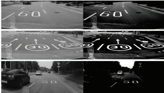
Fig. 4. Grayscale images of ROI (left), and those images of histogram partitioning and stretching (right).
