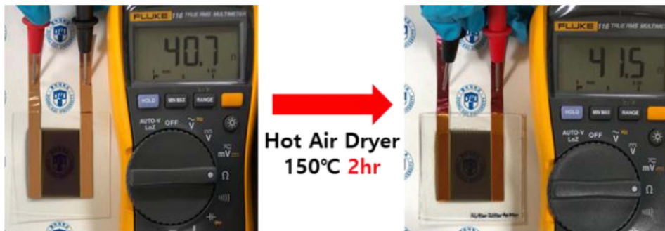
Fig. 2. Comparison of resistance of the deposited substrate after annealing at 150°C for 2 hr.
