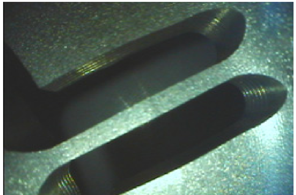
Fig. 8. The original appearance of the spring damper before deformation.
