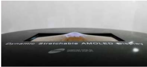
Fig. 2. Image of stretchable AMOLED display paper made by Samsung Display
