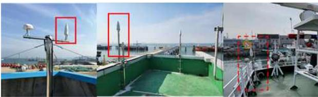
Fig. 1 E-field antenna establishment for eLoran LDC message reception campaign (left: Pyeongtaek differential Loran station, center: Incheon differential Loran station, right: Insung 1-ho)
