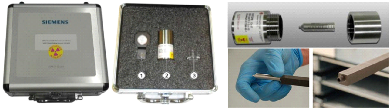
Fig. 2. NIST source set contains 3 parts; 1. Co-57 or Se-75 peaking source 2. Precision Co-57 or Se-75 Calibration source and shield 3. Dose calibrator source holder for positioning calibration source in dose calibrator.
