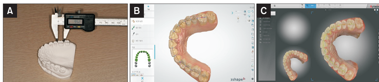
Fig. 2. Model types used for the measurements; (A) manual measuring on a plaster model with a digital caliper (Manual group); (B) measuring the upper arch using Ortho Analyzer software (3Shape®, Copenhagen, Denmark) (LS group); (C) measuring the upper arch using Autolign software (Diorco, Yongin, Korea) (DS group).
